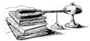
magazine, "a sketch of Henry's primitive telegraph, a dozen years before Morse, reveals the essential components: an electromagnet activated by a distant battery, and a pivoted iron bar that moves to ring a bell."
