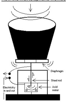
Simplified diagram of Bell's liquid transmitter. The diaphragm vibrated with sound waves, causing a conducting rod to move up and down in a cup of acid water. Battery supplied
